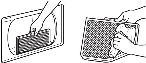
Clean the lint screen before each load. Pull the lint screen straight up. Roll lint off the screen with your fingers. Do not rinse or wash screen to remove lint. Push the lint screen firmly back into place.
