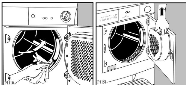
The filter in the inner door must be removed for cleaning.
