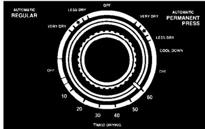
1. **Select a cycle** by turning the Cycle Control Knob either way. Stop when the indicator on the knob's outer ring points to the cycle and setting you want. See pages 7-8 for further cycle information.
