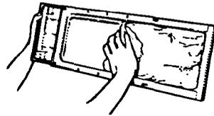
2. Roll lint off the screen with your fingers. Do not rinse or wash the screen to remove lint. Wet lint is hard to remove.
