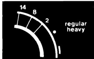
Use for sturdy white and colorfast cottons, and for heavy work clothes. High agitation and spin speeds are designed to help remove heavy soils and spin water from heavy cotton fabrics.
