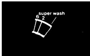
Use as a double wash for heavily soiled loads. Use enough detergent for two washes (SUPER WASH and REGULAR HEAVY).
