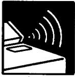
The lint signal (a whistle tone) indicates excessive lint is present on your lint screen or it has a residue buildup. See the "Cleaning the lint screen" section. A full lint screen restricts airflow and reduces drying efficiency. When you hear the signal, stop the dryer and clean the lint screen.
