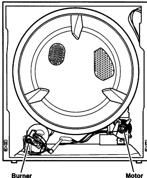
Dryer with front panel removed
