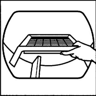
Lower the front so the legs rest on the dryer opening.
