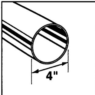
Use 4-inch heavy metal or flexible metal vent. Do not kink or crush flexible metal vent. It must be completely extended to allow adequate exhaust air to flow. Check vent after installation. Refer to your Installation Instructions for proper length requirements of vent.
