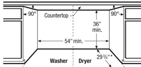
**Side-by-Side Units in Under-Counter Installation**
