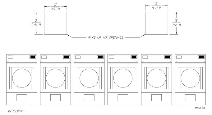
TYPICAL INSTALLATION SHOWING MAKE-UP AIR OPENINGS
