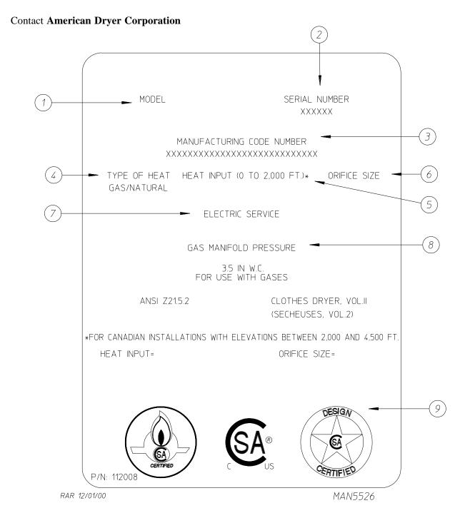
When contacting **American Dryer Corporation**, certain information is required to insure proper service/parts information from **ADC**. This information is on the data label located on the left side panel/wall area behind the control door. When contacting **ADC**, please have the **model number** and **serial number** available.
