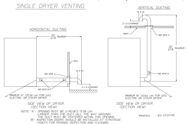
**IMPORTANT:** For extended ductwork runs, the cross section area of the duct can only be increased to an extent. Maximum proportional ductwork runs **cannot** exceed 20 feet (6.09 meters) more than the original limitations of 20 feet (6.09 meters) with two (2) elbows. When the ductwork approaches the maximum limits as noted in this manual, a professional heating, venting, and air conditioning (HVAC) firm **should be** consulted for proper venting information.
