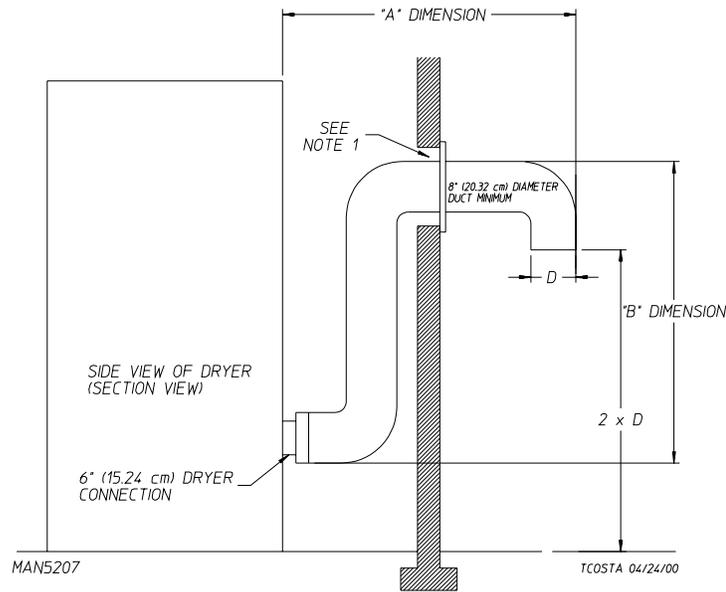
NOTE 1: OPENING MUST BE 2-INCHES (5.08 CM) LARGER THAN THE DUCT (ALL THE WAY AROUND). THE DUCT MUST BE CENTERED WITHIN THIS OPENING.
