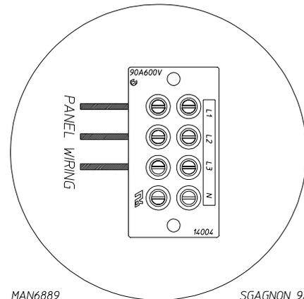
The neutral will only be used on 4-wire service. This is typical for 380-416V, 50 Hz.
