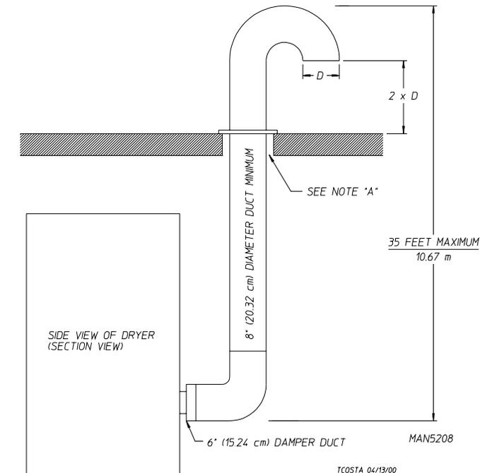
NOTE A: OPENING MUST BE 2-INCHES (5.08 cm) LARGER THAN THE DUCT (ALL THE WAY AROUND). THE DUCT MUST BE CENTERED WITHIN THIS OPENING.
