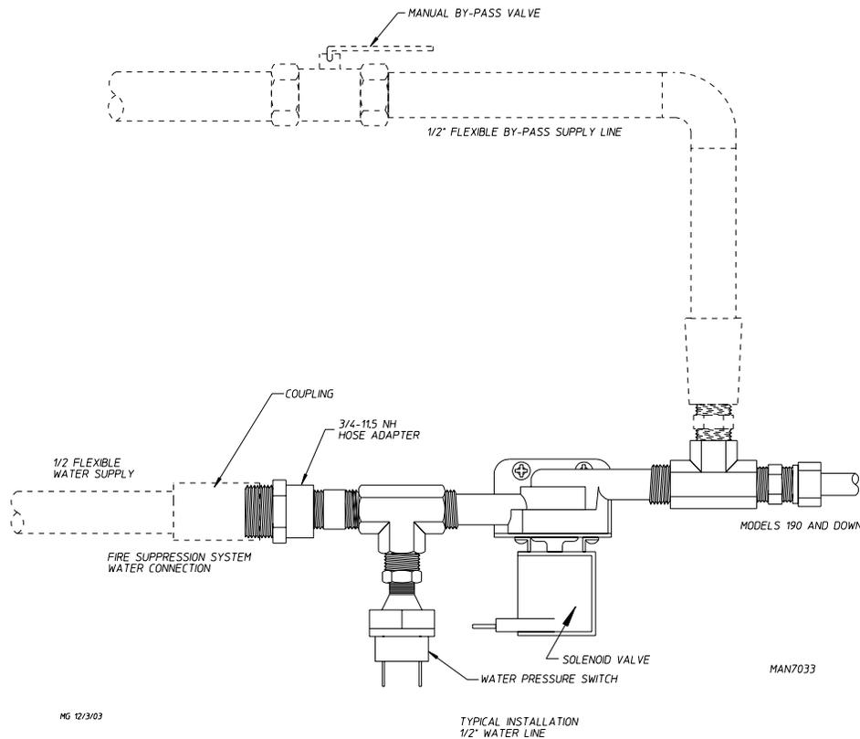
**WARNING:** If the water in the supply line or water solenoid valve freezes, the S.A.F.E. system **will be** INOPERATIVE!!
