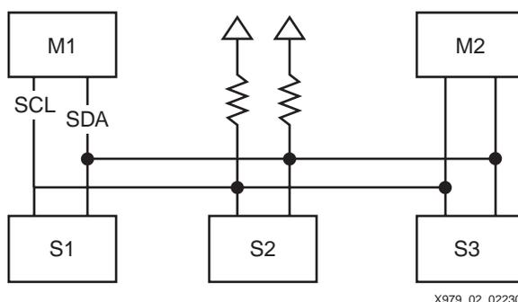
**Figure 2: IIC Bus**
