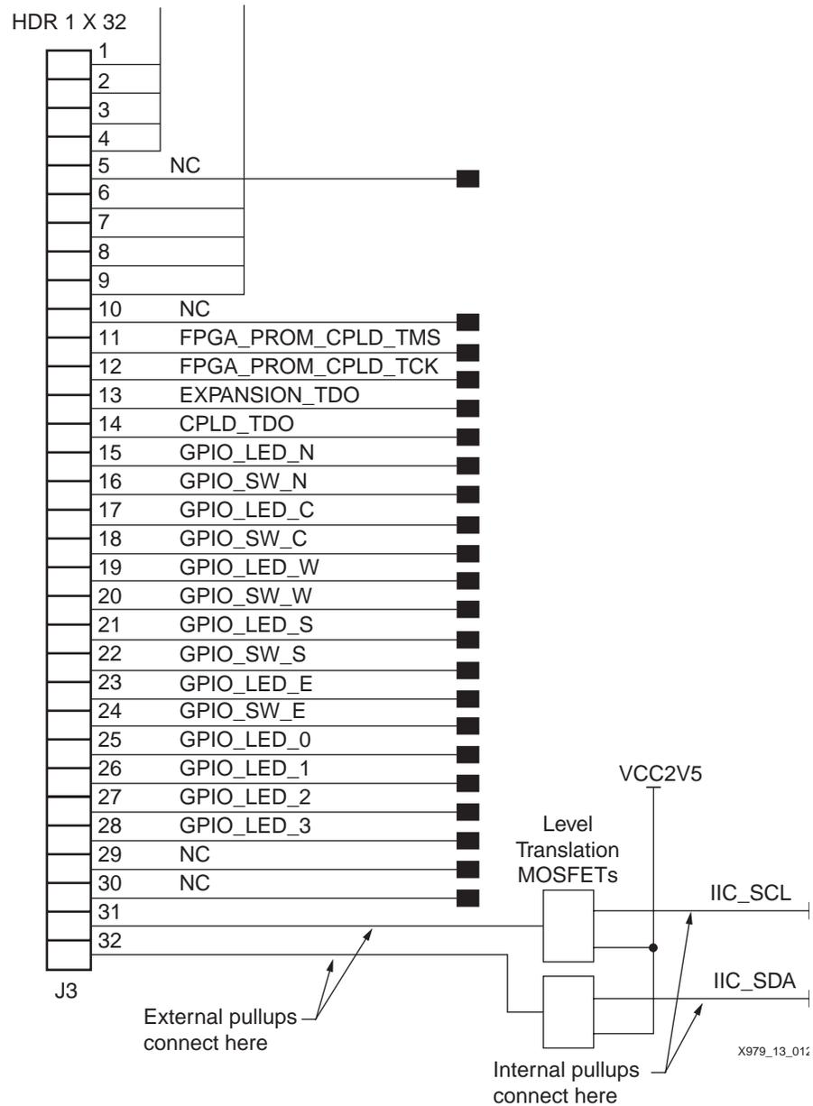
Figure 13: Expansion Header
