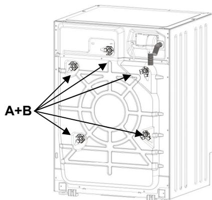
1. Undo **all** the screws with a 10 mm spanner.
