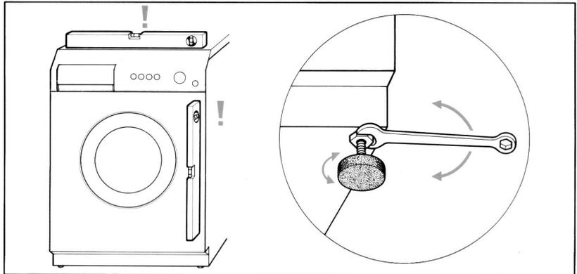
3. On appliances with **adjustable rear feet**, note that the rear of the appliance rests on skids and not on the feet. Before inserting the appliance into its place between the kitchen units, check that the rear feet are screwed fully in to prevent damage as the appliance is shifted into position.
