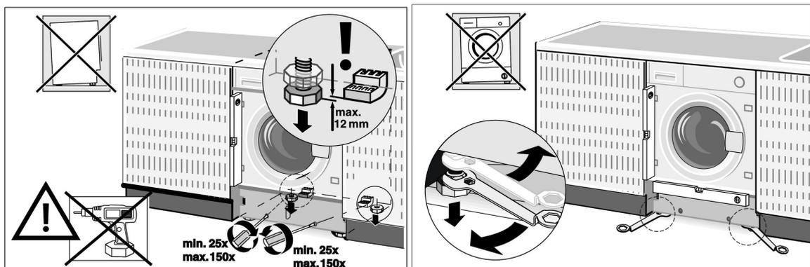
The water intake and drain hoses can be fitted pointing to the left or right for effective installation.
