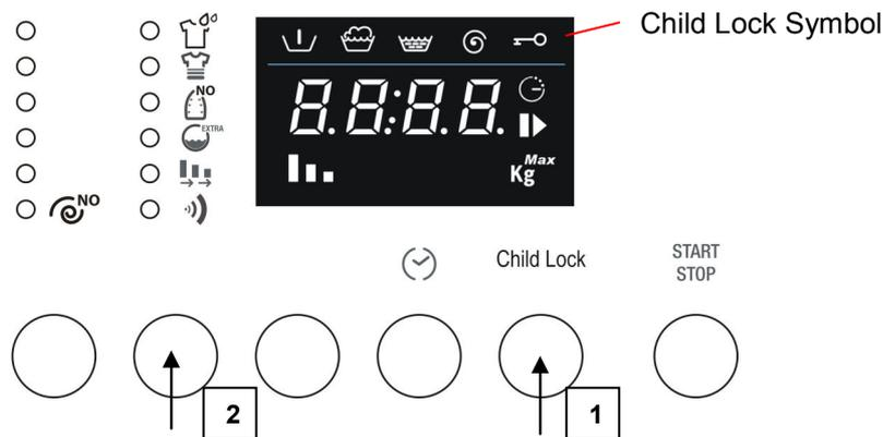
2. To activate the Child Lock Function, press the Child Lock (1) button and hold it down. Also press the Options selection (2) button within 3 seconds.
