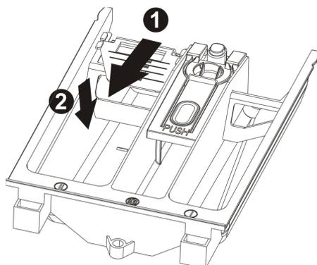
Following the recommendations in the "Programmes Table" supplied with this manual, place the detergent and any additives in the drawer before the start of the programme.
