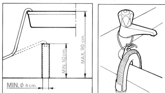
2. In all cases, check that the end of the drain hose is securely fixed to prevent the repulsive force of the water from pushing it out of place.
