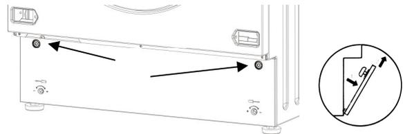
Free-Standing Model – Insert a small screwdriver through the slits in the front of the plinth, then apply upward leverage with the screwdriver to release the top of the plinth from the cabinet.
