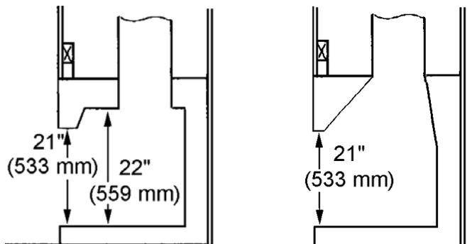
**Do not face seal over chimney cooling air system.**
