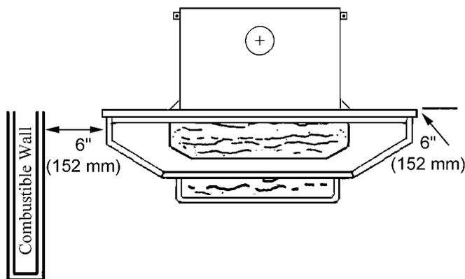
For installation with a combustible mantel or top trim, Part #16101 deflector must be installed.
