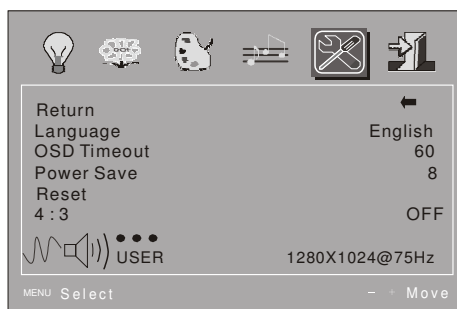
Display mode:when setting OFF,it is display mode,whensettingON, it will be 4:3 display mode
