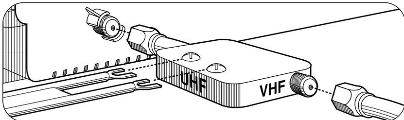
**If your antenna system has two sets of twin 300-ohm leads,** you must obtain a combiner (available at your local electronics store). Place one set of twin leads underneath the screws on the combiner and tighten the screws. Do the same with the other set of twin leads. Press the cable from the combiner onto antenna terminal on the back of your TV.
