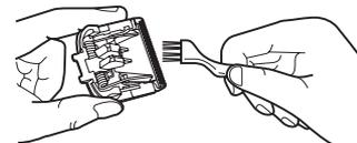
3. Brush any hair trimmings out from between the stationary blade and the moving blade while pressing down the cleaning lever to raise the moving blade.
