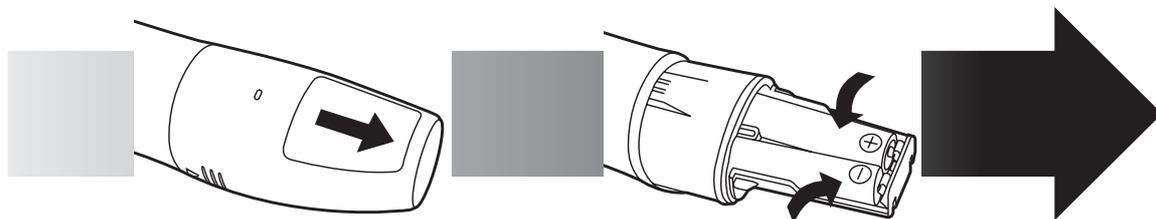
1. Slide the switch on the main body downwards to turn off the trimmer.
