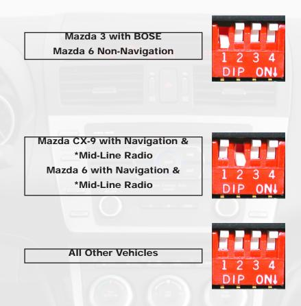
\*The Mid-Line Radio will have a small color LCD in the middle of the face of the radio and will not have a seperate text display.
