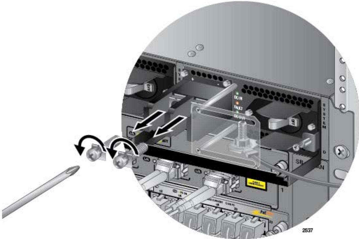
Figure 127. Removing the Terminal Screws
