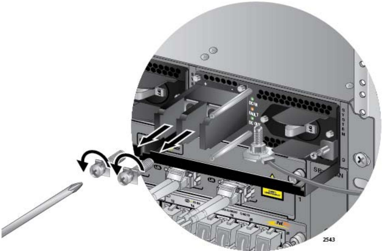
Figure 135. Removing the Terminal Screws
