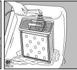
Also clean the outside, removing all fluff. Clean the rubber seal round the porthole door and the seal of the condenser in the inner door with a damp cloth.
