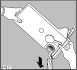
The reservoir must be re-inserted correctly.
