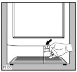
To pull out the condenser, first turn the two red stops downwards as shown below and then remove the condenser unit holding it at the handle.
