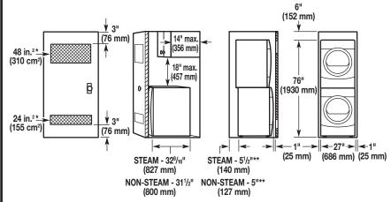
For dryer on pedestal; cabinet installation, with a door, the minimum ventilation openings in the top are required.
