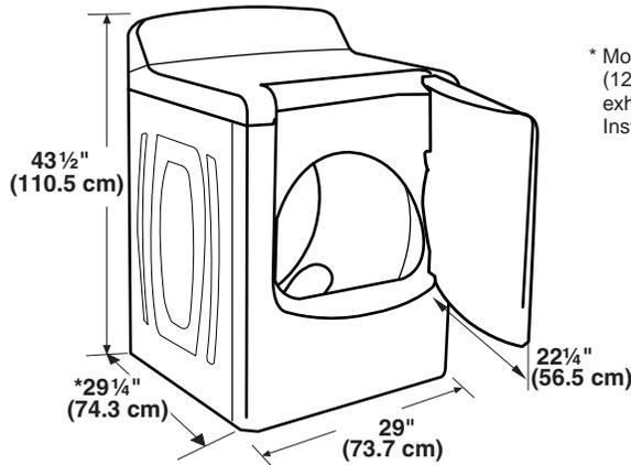
\* Most installations require a minimum 5" (12.7 cm) clearance behind the dryer for the exhaust vent with elbow. See Installation Instructions, "Venting Requirements."
