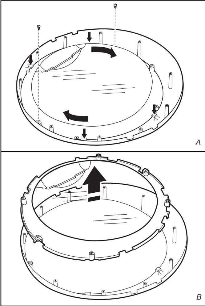
Using a Phillips screwdriver, remove the 2 screws from the outer window retainer and rotate the outer window assembly clockwise until the square notches line up with the 4 tabs on the trim ring indicated with arrows in the figure A above. Then lift out the outer window and retainer up and off the trim ring and set aside (B).
