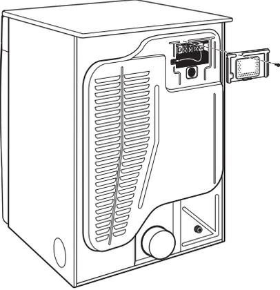
Remove hold-down screw and terminal block cover.
