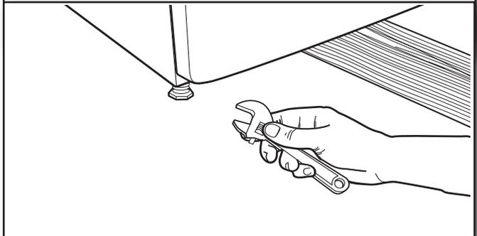
If dryer is not level, prop up using a wood block, use wrench to adjust legs up or down, and check again for levelness. Once dryer is level, make sure all four legs are snug against the floor and dryer does not rock.
