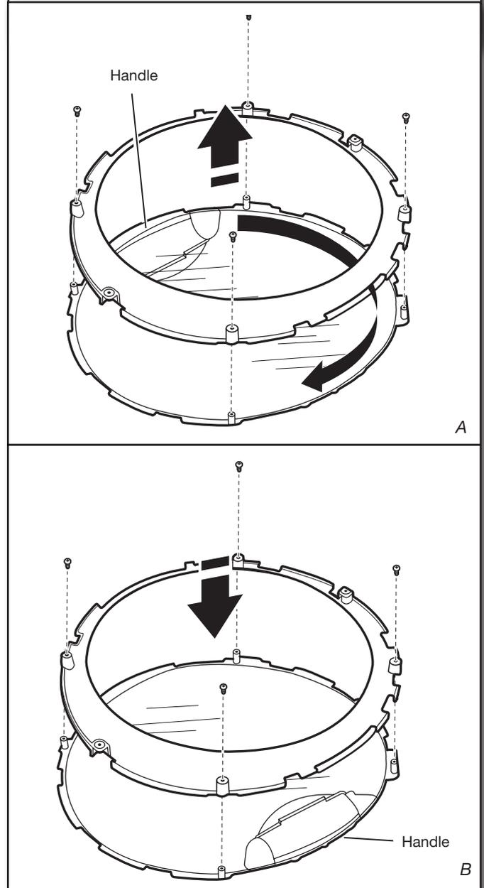
Using a Phillips screwdriver, remove the 4 screws from the outer window retainer and lift off the trim ring off the window (A). Rotate trim ring 180° and secure with the 4 screws removed earlier (B).
