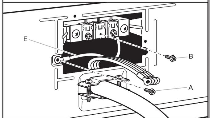
Remove center, silver-colored terminal block screw (B). Remove neutral ground wire (E) from green external ground conductor screw (A).
