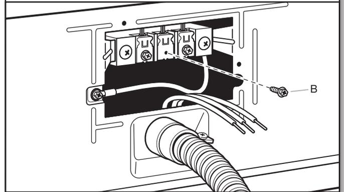
Remove center terminal block screw (B).
