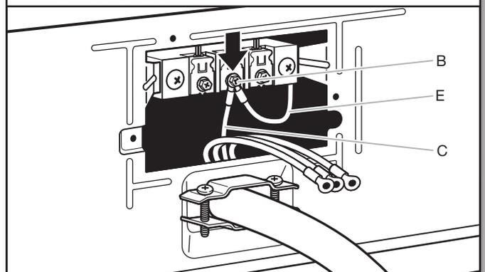
Connect neutral ground wire (E) and neutral wire (white or center) (C) of power supply cord under center terminal block screw (B). Tighten screw.
