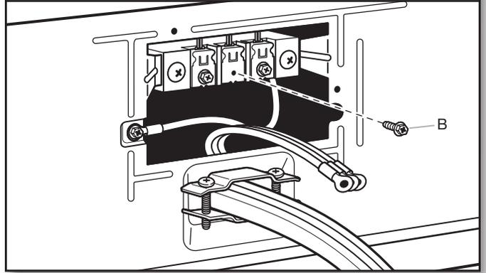
Remove center terminal block screw (B).
