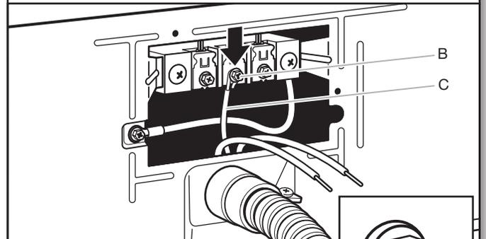
Place hooked end of neutral wire (white or center) (C) of direct wire cable under center terminal block screw (B), hook facing right. Squeeze hooked end together. Tighten screw.
