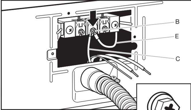
Connect neutral ground wire (E) and place hooked end (hook facing right) of neutral wire (white or center wire) (C) of direct wire cable under center screw of terminal block (B). Squeeze hooked ends together and tighten screw.
