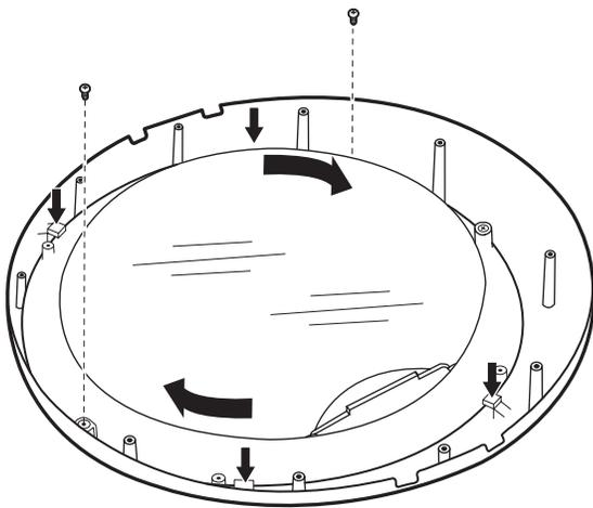
With the edge with 2 notches at the top, align the notches on the outer window assembly with the tabs on the trim ring and lower into place as shown in figure A.
