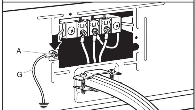
Connect a separate copper ground wire (G) under the green external ground conductor screw (A) to an adequate ground. Finally, reinsert tab of terminal block cover into slot of dryer rear panel. Secure cover with hold-down screw. Now, go to Venting Requirements.
