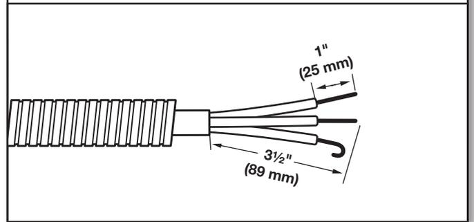
Direct wire cable must have 5 ft. (1.52 m) of extra length so dryer may be moved if needed.
