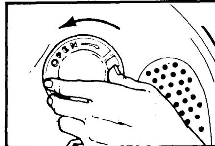
4. Replace the light bulb cover and lock it in place by turning counterclockwise.
