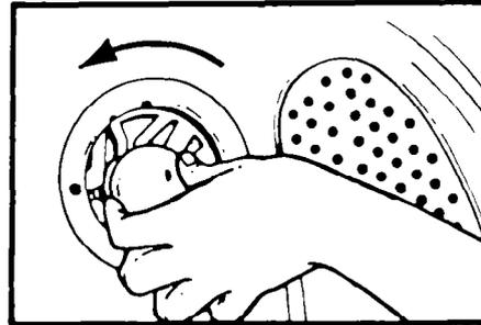
2. Remove the light bulb by turning it counterclockwise.
