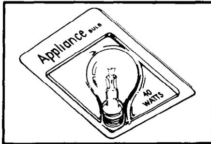
3. Replace the bulb only with a **40-watt appliance bulb** from most hardware, grocery or variety stores.
