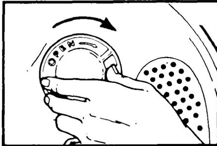
1. Open the dryer door and remove light bulb cover by turning it clockwise.
