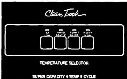
2. **Press a temperature selection** which matches the type of fabric being dried. The indicator will appear over the temperature selection you have chosen.
