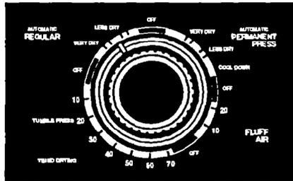
1. **Select a cycle** by turning the Cycle Control Knob either way. Stop when the indicator on the knob's outer ring points to the cycle and setting you want. See pages 6-8 for further cycle information.
