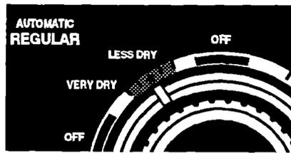
**Use AUTOMATIC PERMANENT PRESS** to dry permanent press, knits and other synthetic items. The load tumbles without heat during the last 10 minutes. This helps keep wrinkles from setting in and makes the load easier to handle.
