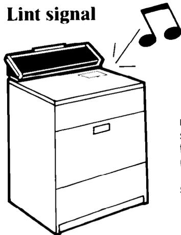
Clean lint screen **before each load**. If you neglect to clean your lint screen, the signal will sound. The (whistle tone) signal lets you know the air flow is being restricted. Restricted air flow reduces drying efficiency.
