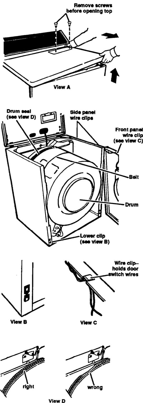
If your dryer is gas and has a full front panel, remove front panel as follows:
