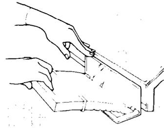
To remove the screen, open the lid and pull the screen straight out. Roll the lint off the screen with your fingers.
