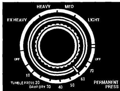
1. **Select a cycle** by turning the Cycle Control Knob either way. Stop when the indicator on the knob's outer ring points to the cycle and time you want. See pages 6-9 for further cycle information.
