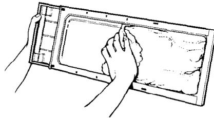
2. Roll lint off the screen with your fingers. **Do not** rinse or wash the screen. Wet lint is hard to remove.
