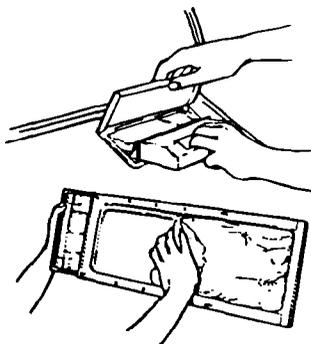
2. Roll lint off the screen with your fingers. Do not rinse or wash the screen to remove lint. Wet lint is hard to remove.
