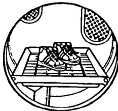
1. Fit rear legs of the rack into indentations in the back wall of the dryer.
