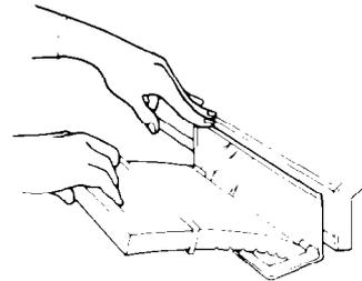
To remove the screen, open the lid and pull the screen straight out. Roll the lint off the screen with your fingers. **DO NOT rinse the screen or wash it.** Wet lint is hard to remove.
