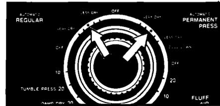
For the first few loads, set the Control Knob to point to an ✱ in either automatic cycle. When the dryer stops, feel the dried items.
