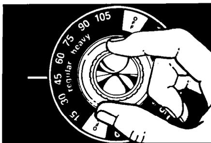
Turn the Control Knob either way to point to the cycle and time setting you want.
