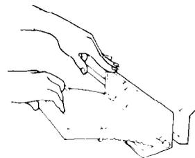
*To remove the screen, open the lid and pull the screen straight out. Roll the lint off the screen with your fingers.*
