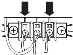
5. Tighten strain relief screw.
