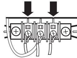
4. Tighten strain relief screws.
