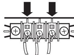
4. Tighten strain relief screws.
