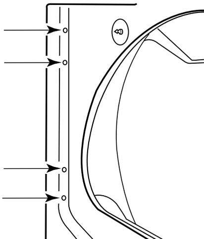
6. Install 4 plastic plugs into screw holes in the dryer left where the hinges were removed in Step 4.
