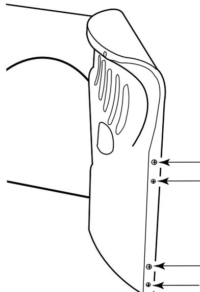
4. Install the 2 hinges to the front panel of the dryer using 4 screws. Use the non-slotted side to attach the hinge to the front panel.
