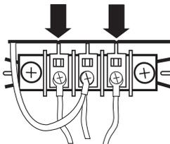
5. Tighten strain relief screws.
