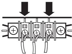
4. Tighten strain relief screw.
