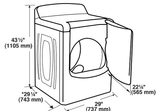
\*Most installations require a minimum 5" (127 mm) clearance behind the dryer for the exhaust vent with elbow. See "Venting Requirements."
