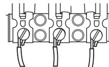
1. Loosen or remove center terminal block screw.
