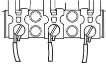
1. Locate the neutral ground wire inside the dryer cabinet, behind the external ground conductor screw. Remove this wire.
