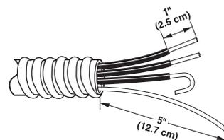
When connecting to the terminal block, place the hooked end of the wire under the screw of the terminal block (hook facing right), squeeze hooked end together and tighten screw. See example below.
