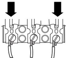
6. Replace the terminal block cover on the back of the dryer.
