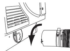
5. Make sure the exhaust vent is placed inside the exhaust hood and then secured to the exhaust hood with a 4" (10.2 cm) vent clamp.
