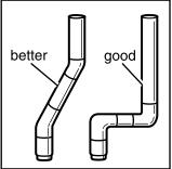
the exhaust vent. Use the fewest number of elbows and turns. Allow room when using elbows or making turns. Bend vent gradually to avoid kinking.
