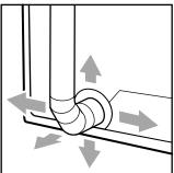
• Exhaust from the rear of the dryer: The exhaust vent can be routed up, down, left, right, or straight out the back of the dryer. Space requirements are listed in your Installation Instructions.
