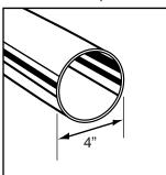
Use 4-inch heavy metal or flexible metal vent. Do not kink or crush flexible metal vent. It must be completely extended to allow adequate exhaust air to flow. Check vent after installation. Refer to your Installation Instructions for proper
