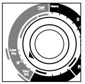
Depending on your model, the Automatic cycle uses either the electronic ACCUDRY™ system or the automatic DRY-MISER® control that senses the moisture in the load and shuts off the dryer when the selected dryness is reached.
