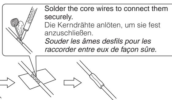
Solder the core wires to connect them securely.
