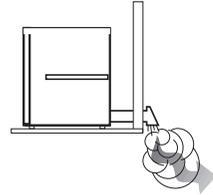
2. Use 4" diameter rigid metal duct. Tape all joints, including at the dryer.
