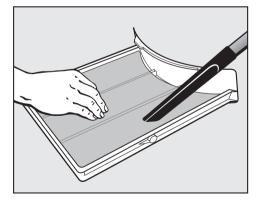
Wipe the lint off the filter with your hand (do not use any sharp objects!) or use a vacuum cleaner with the nozzle attachment (supplied with the vacuum cleaner).
