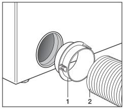
■ Install the exhaust hose/pipe, **2**, with the connector, **1**, to the dryer.
