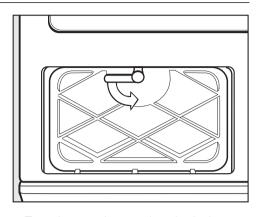
Turn the condenser door lock down and remove the door.
