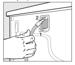
■ Unclip the drain hose, **1**, and pull it off the holder **2**.
