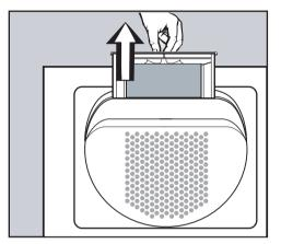
■ Open the door and remove the lint filter by gently lifting it upwards.
