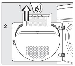
Open the door and pull the fluff filter
