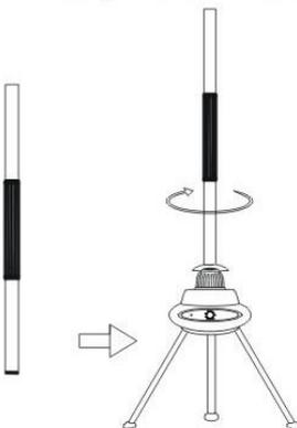
4. Insert the hanger into the upper supporting tube and then pull the aluminum hangers down into the level position.
