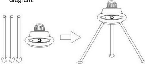
2. Connect the three tubes that form the support arm by screwing them in to each other
