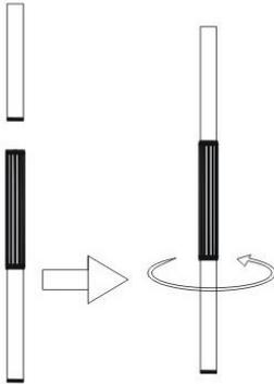
3. Fit the water-proof plate onto the lower supporting tube and then attach the lower supporting tube onto the motor body by screwing it in a clockwise direction.
