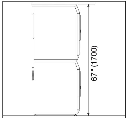
The Miele dryer can be installed as part of a washer-dryer stack in combination with a Miele washer. An appropriate "stacking kit" available from Miele is required. Installation of the stacking kit must be completed by a Miele Service Technician.
