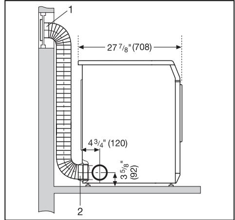
**1** Window connection (installed in an "plexiglass" pane)
