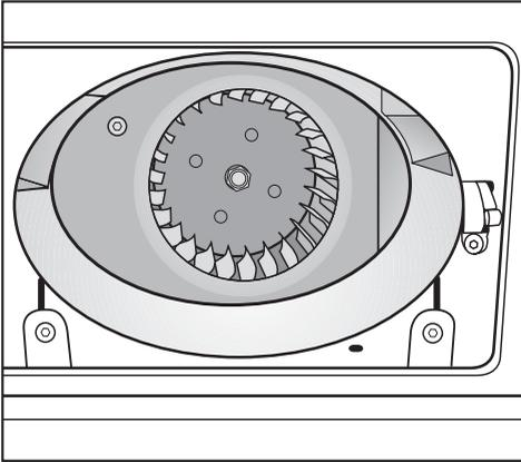
The impeller in the dryer interior can become clogged with detergent residues or lint.
