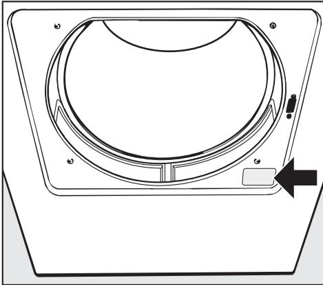
The **PC** indicator allows a service technician to check and update the drying programs.
