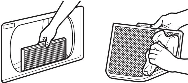
Clean the lint screen before each load. Pull the lint screen straight up. Roll lint off the screen with your fingers. Do not rinse or wash screen to remove lint. Push the lint screen firmly back into place. For additional cleaning information, see "Dryer Care."
