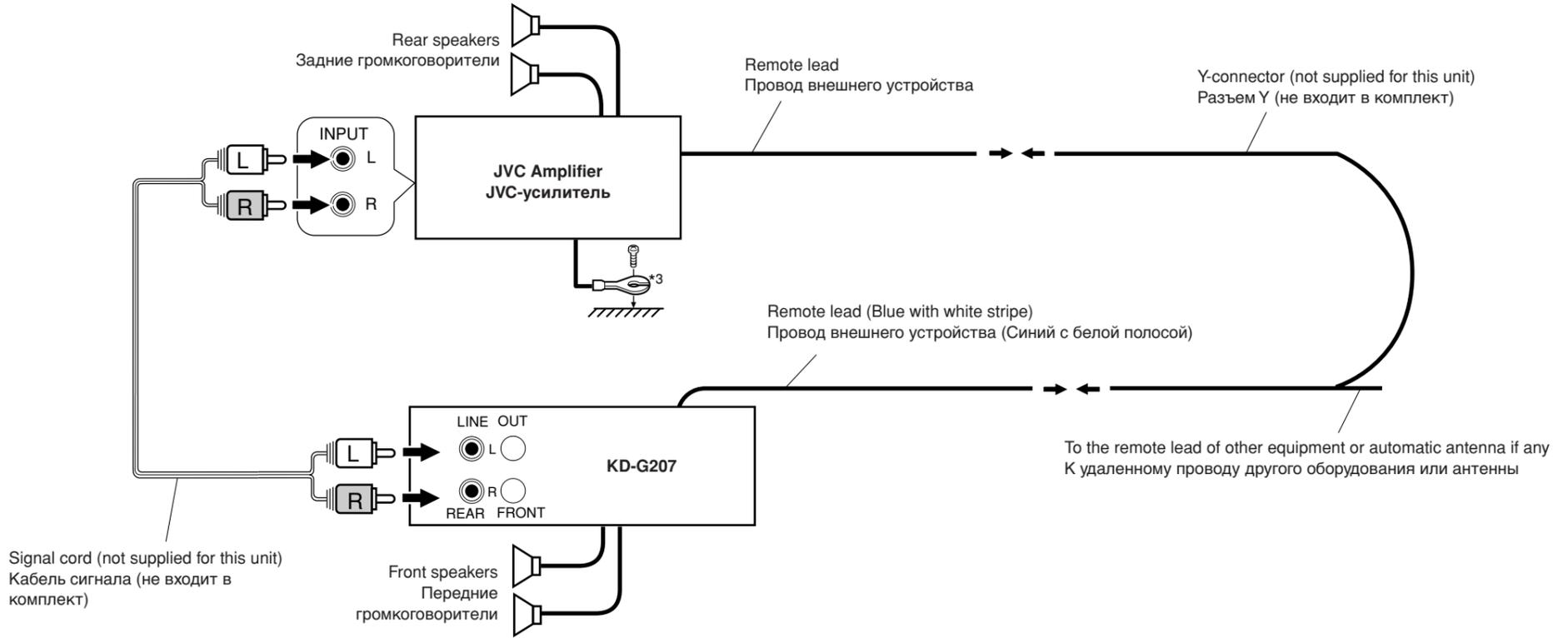
\*3 Firmly attach the ground wire to the metallic body or to the chassis of the car—to the place not coated with paint (if coated with paint, remove the paint before attaching the wire). Failure to do so may cause damage to the unit.
