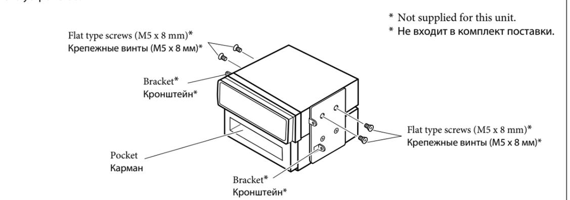
**Note** : When installing the unit on the mounting bracket, make sure to use the 8 mm-long screws. If longer screws are used, they could damage the unit.
