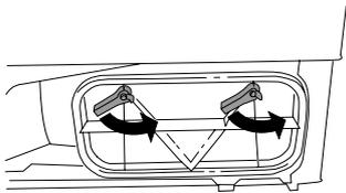
4. Remove the condenser and rinse the lamellas clean using a hand shower, for example. Do not poke around in the lamella springs, as you may damage the condenser. Do not use pointed metal objects during cleaning.
