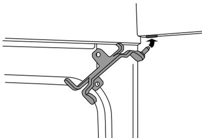
**13.** Secure the hinge attachment using the screws in the sequence shown in the picture.
