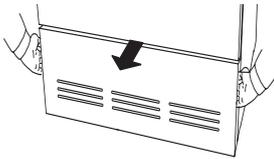
3. Open the condenser panel by turning the two knobs anticlockwise.
