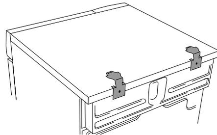
3. Attach the plastic cups that will hold the tumble dryer's front feet to the washing machine's top cover. This is essential, as once the tumble dryer's feet are resting in the plastic cups you know the dryer is correctly positioned on the washing machine.
