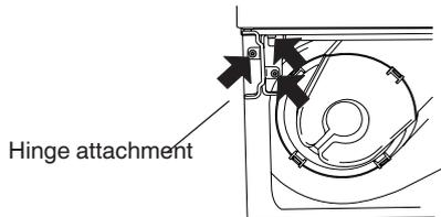
3. Move the hinge pin. For right hanging, the hinge attachment must then be turned upside down.
