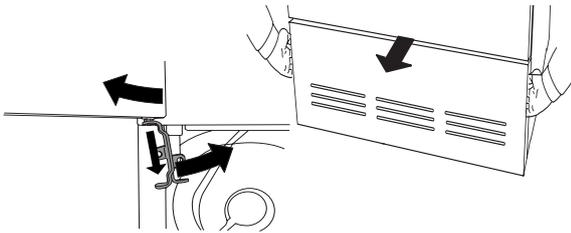
2. Angle the lower edge of the door out to the left while turning the hinge attachment as indicated by the arrows.
