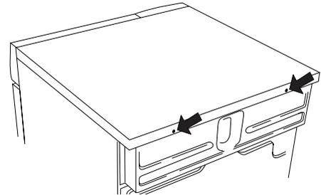
2. Secure the anti-tilt device using the screws as shown in the picture.
