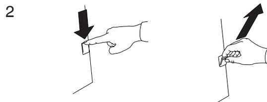
8. Insert the door magnet in place of the cover washer.
