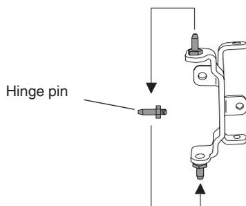
4. Then move the hinge pin in the panel's lower edge.
