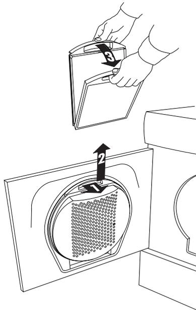
3. Open the filter and remove the fluff from all sides by hand. Use a soft dry cloth to remove any coating.
