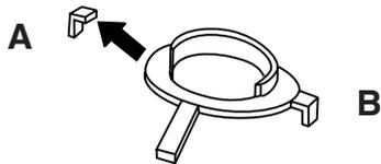
4. Fit the plastic cups so that the “tags” marked with arrows are against the front edge of the cover and side edge and press firmly onto the cover. Then break off the remaining tags.
