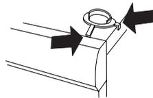
5. Push the tumble dryer in under the metal angles, keeping the front edge raised 1 - 2 cm.
