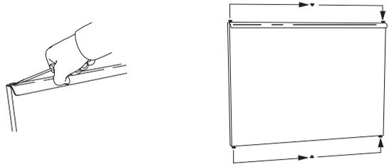
6. Unscrew the two screws on the sides of the door, around five millimetres, to allow the door magnet and cover washer on the inside of the door to be removed.
