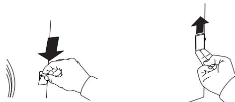
**9.** Insert the cover washer in place of the door magnet.
