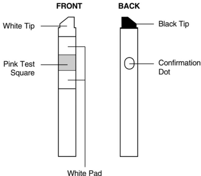
**Black Tip** helps the meter detect that the strip has been inserted properly.
