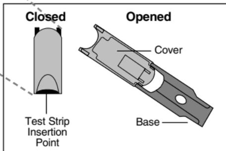
The cover protects the lens area and the base holds the SureStep Test Strip.
